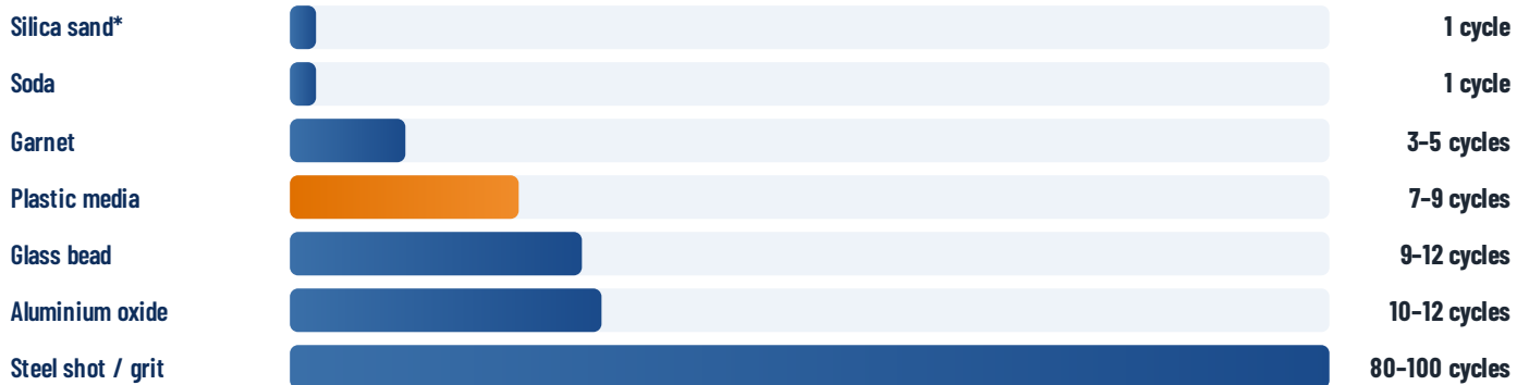
Figure 1 · Media life in recovery cycles (PanBlast™ abrasive breakdown reference data; plastic media ≈13% breakdown per cycle). Dry ice: zero cycles by definition — the media sublimates. *Silica sand shown for reference only; prohibited for blasting in many jurisdictions.
