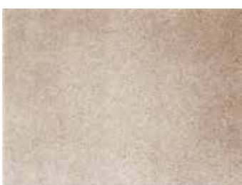
Condition A Blasted to Sa3
