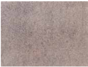
Condition A Blasted to Sa2
