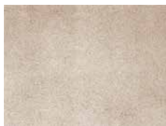
Condition B Blasted to Sa3
